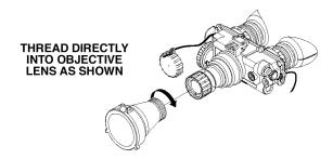
Figure 2-26. 3X Magnifier Installation without LIF
